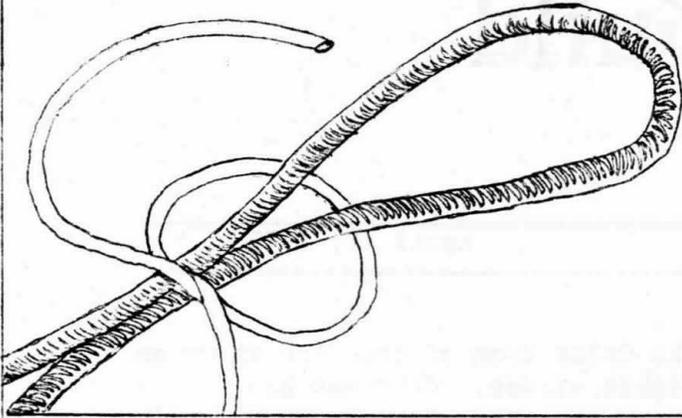
Step 1. Make a loop in the line to be siezed. Tie an overhand knot with the siezing line, leaving enough line to work with later.
