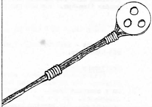
Step 6. Slide the sieze to where it is needed, insert Deadeye and pull the excess line through the sieze. until the Deadeye is captured. Cut excess line.
