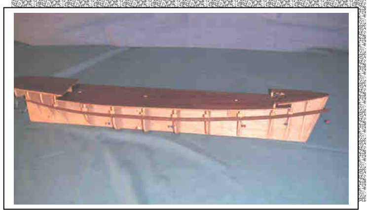
Chuck Peabody's CUTTY SARK. Deck complete. First plank on.
