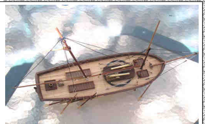
Hawkins Gunboat from above, showing the unique gun system. Photo by John Wickman
