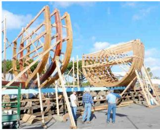
San Salvador framing as of 21 Dec 2011. Frames are made of Carolina's Live Oak, held together treenails only. Below blue expoxied keel there will be lead balast weighing 6000 pounds each, about 10 or 60,000 pounds balast. Planking will be  $2\,1/4$ " thick. Fir above the water line and a South American mohagany type below the water line. John Wickman
