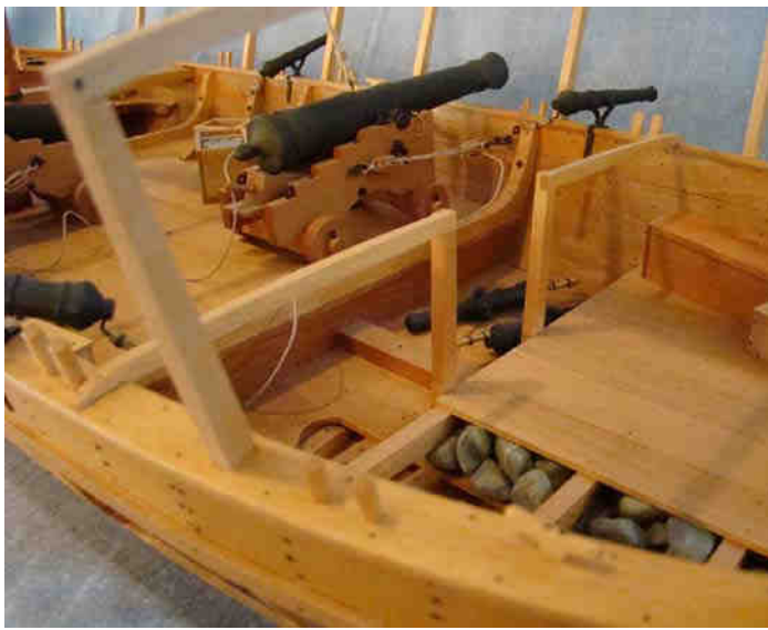
Above: Starboard 9 pounder, swivel guns and aft platform (exposed showing ballast to compensate for forward 12 # gun).
