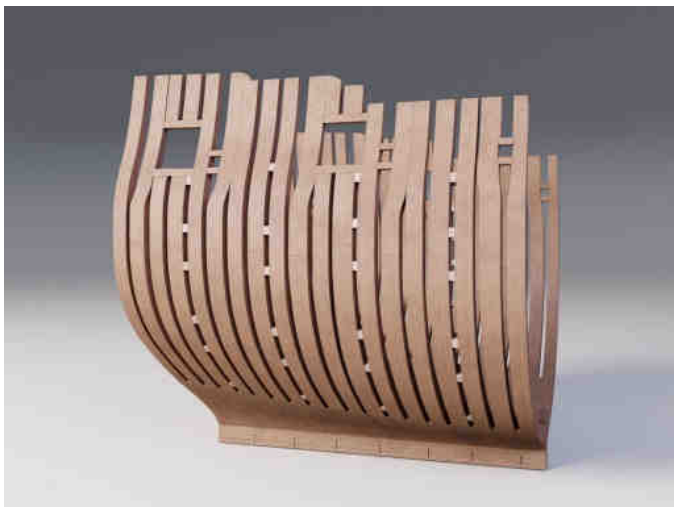
Chuck Passaro's PEGASUS Cross-Section: Structural Framing.
