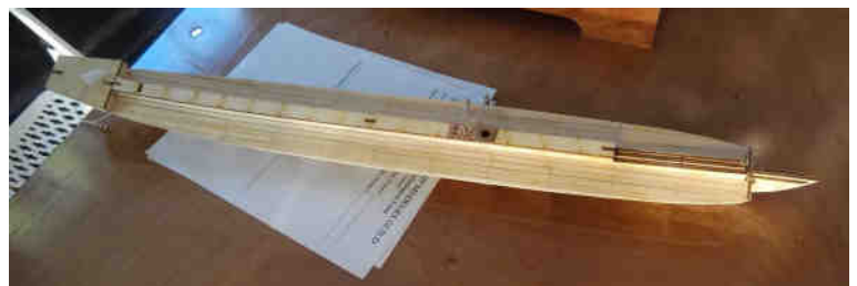
Photo shows the first layer of deck planking.
