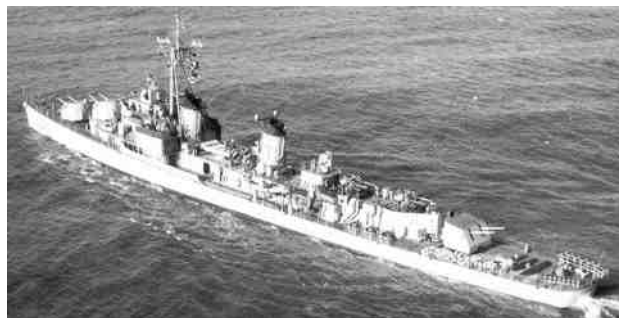
BRINKLEY BASS in the mid-1950s with tripod mast for heavier radars and 3"/50 gun mounts replacing 40mm and 20mm AAW batteries from http://www.navsourc.org/archives/05/pix1/0588712.jpg
