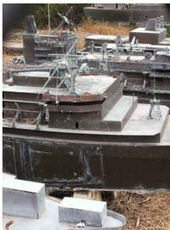
Notice the antenna test equipment on these brass models
