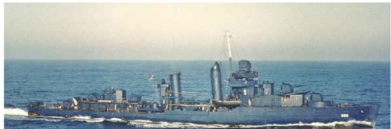
Editor addition: USS DRAYTON (DD-366) showing Measure 21 blue camouflage in color. From Measure 21 (shipcamouflage.com) an online database.
