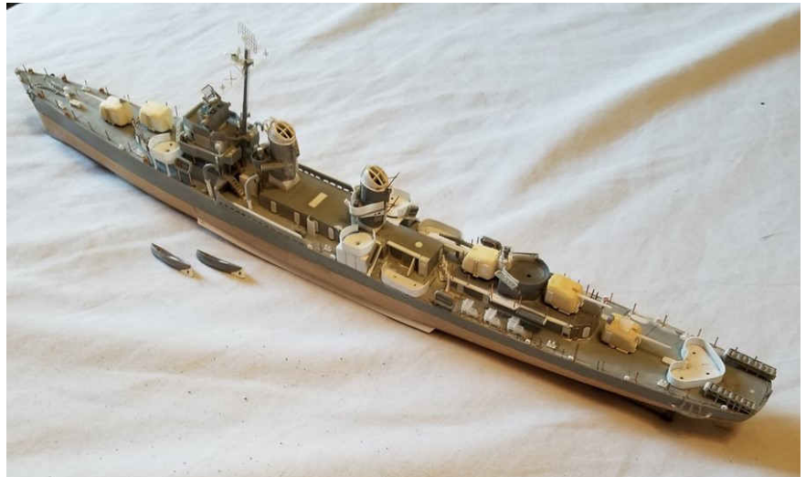
Figure 9 - USS McDERMUT model in progress from the port quarter. Note the white plastic hand fabricated and yellow resin cast parts, brass stanchions, ladders, and radars.
