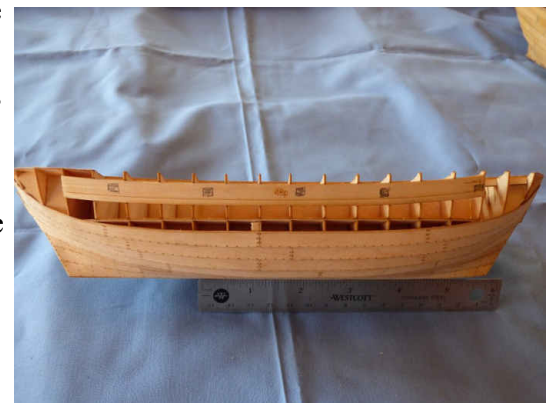
Left - PIC4: Locating the bulkheads vis-à-vis the marks on the hull.
