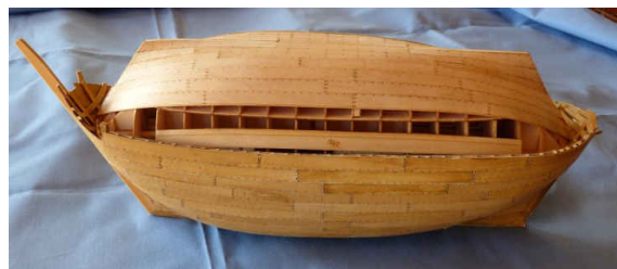
Left - PIC4: Locating the bulkheads vis-à-vis the marks on the hull.
