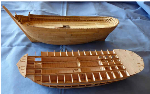
Above - PIC3: One problem-at the point I made this decision, the ship was decked over and I was not sure where the bulkheads were. Solution: Compare the undecked Woodydog to the decked Cardydog to determine bulkhead location and proceed accordingly.
