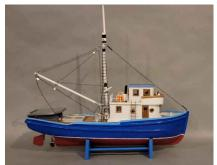
New member **Art Arroyo** debuted in a big way with his scratch built model of the tuna boat *Suzanna II*. Built from plans, his model is crafted from basswood and is ballasted with shotgun shot. Capable of radio control, the model features a removable wheelhouse to access the machinery. He is also looking into
