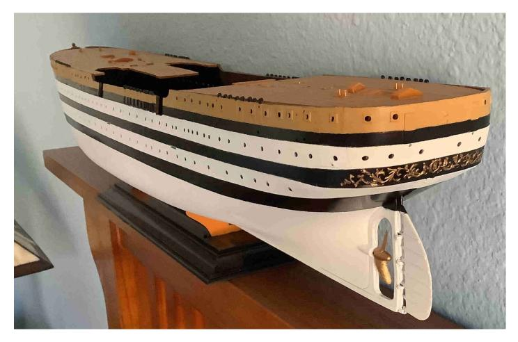
A common problem with large plastic models is hull twist, and this kit was no exception. Don turned to conventional plastic cement to join the halves, then clamped along the keel and bow. He also reinforced the keel join with CA glue. The combination worked and the hull is now aligned and true.
