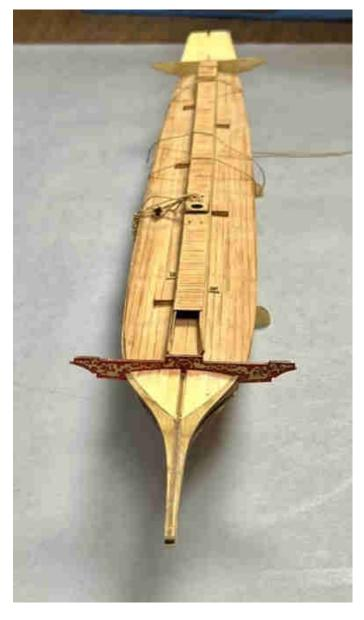
Don Dressel brought in a Battle of Lepanto galley project that is putting up an epic fight of its own. Building a model with such a narrow aspect ratio is challenging enough, but the wood planking twisted on a moist day, so Don re-wet the model, put on a Chubby Checker record, and braced the model for two months to counter the twist. Careful examination, though, still shows a slight mis-alignment between bow and stern, though.
