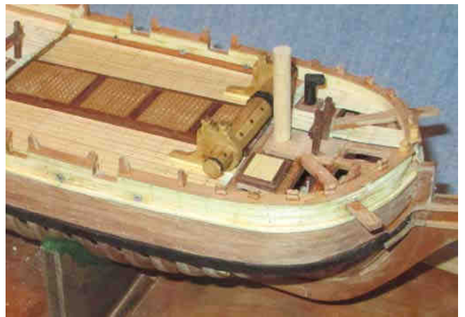
Catheads, caprails and posts installed. The windlass was made from a Chuck Passaro kit.
