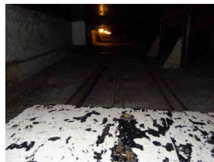
A pull cart on rails gives access to the bilge area on each side of the keel.
