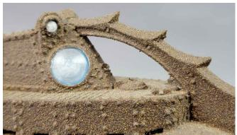
Glenn Clausson brought in a 3D home printed Verne *Nautilus* from the Disney movie design. The model was printed in sections, which took several hours each, for a total of 14 hours. This example was his third attempt. The printing size (scale) is entirely adjustable. The printing material is PLA plastic, a corn-based formulation.
