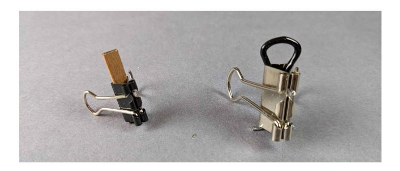
Chuck Seiler brought in a set of "planking clamps," repurposed office binding clips that are useful in holding individual planks onto bulkheads.
