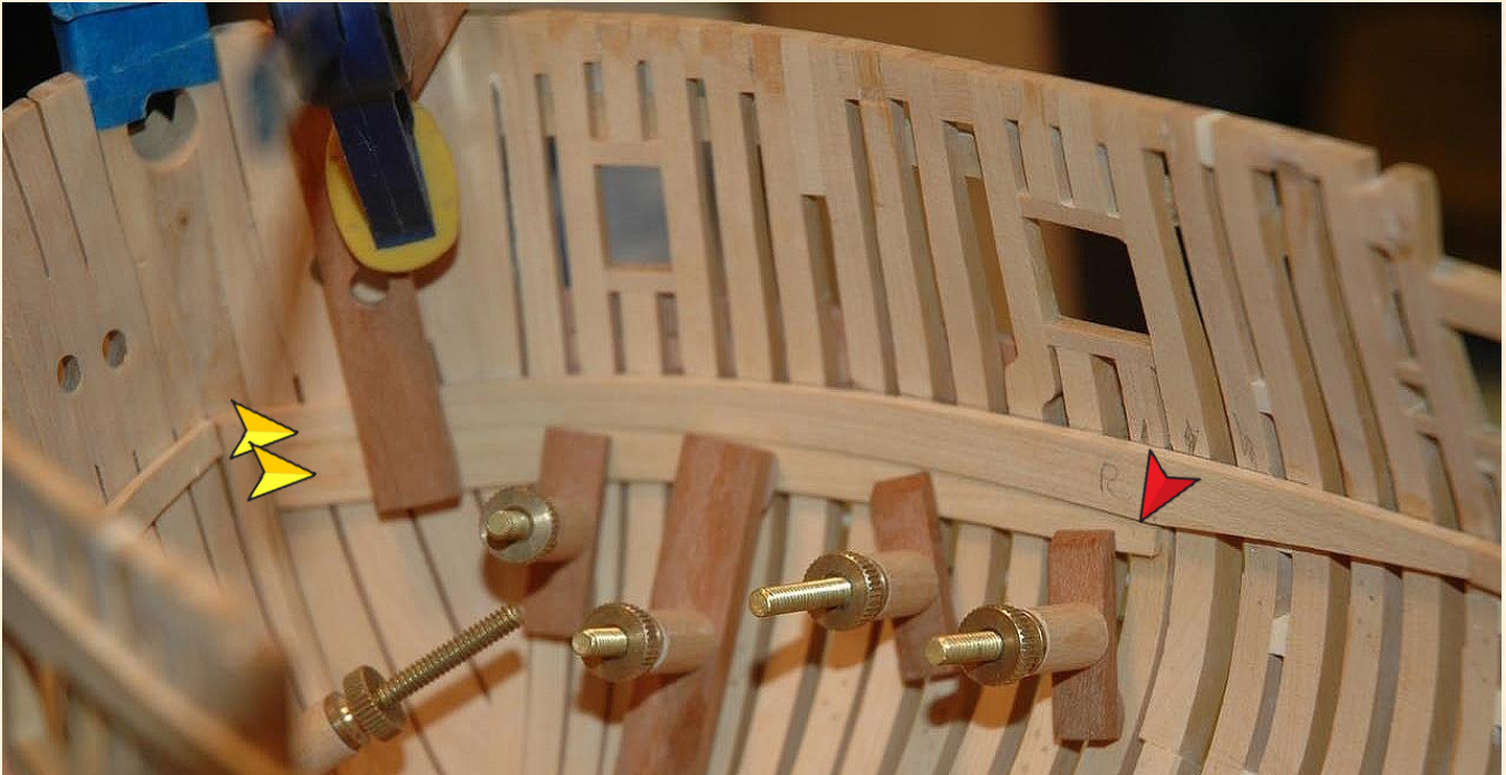
Figure 49 — upper deck clamp installation using top and butt planking
