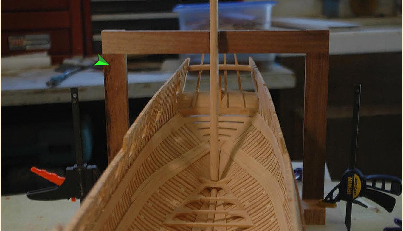
Figure 54 — gantry jig holding mizzen mast (dowel) in place
