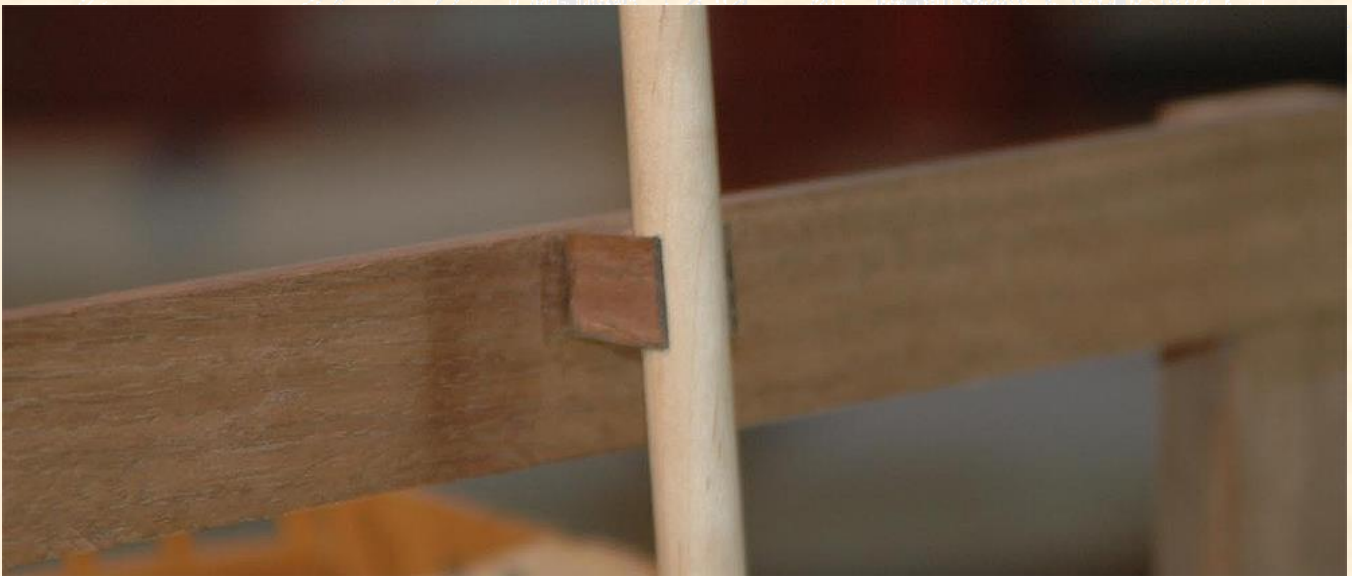
Figure 55 — gantry jig clip used to hold the dowel
